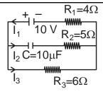
In steady state there will be no current in branch of capacitor, so no voltage drop across  $R_2 = 5\Omega$
