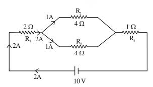
$$R_{eq} = 2\Omega + 2 \Omega + 1 \Omega = 5 \Omega$$
